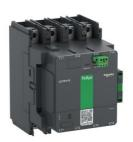
High power contactor, TeSys Giga, 4 pole (4NO), AC-1 <=440V 275A, standard version, 100...250V wide band AC/DC coil
