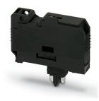
Fuse plug, Prior to replacing the cartridge fuse, disconnect the fuse connector from the basic terminal block., nominal current: 10 A, connection method: Plug-in connection, fuse type: G / 6,3 x 32, mounting type: Plug-in mounting, color: black
