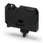
Fuse plug, Prior to replacing the cartridge fuse, disconnect the fuse connector from the basic terminal block., nom. voltage: 630 V, nominal current: 10 A, connection method: Plug-in connection, fuse type:  $G / 6.3 \times 32$ , mounting type: Plug-in mounting, color: black
