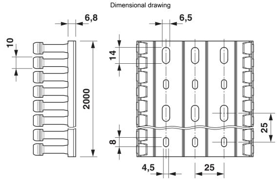
Base perforation according to DIN EN 50085
