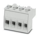
PCB connector, nominal cross section: 2.5 mm², color: light grey, nominal current: 16 A, rated voltage (III/2): 320 V, contact surface: Tin, type of contact: Socket, number of rows: 1, number of positions: 4, product range: MSTBT 2,5 HC/..-STP, pitch: 5 mm, connection method: Screw connection with tension sleeve, conductor/PCB connection direction: 0 °, locking clip: - Locking clip, plugin system: COMBICON MSTB 2,5 HC, locking: without, mounting: without
