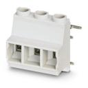
PCB terminal block, nominal current: 24 A, rated voltage (III/2): 630 V, nominal cross section: 2.5  $\,$  mm², number of rows: 1, number of positions per row: 3, product range: MKDSO 2,5 HV/..-R, pitch: 7.5 mm, connection method: Screw connection with tension sleeve, mounting: Wave soldering, conductor/PCB connection direction: 0 °, color: light grey, Pin layout: Linear pinning, Solder pin [P]: 3.5 mm, number of solder pins per potential: 1. Product with pin output on right side
