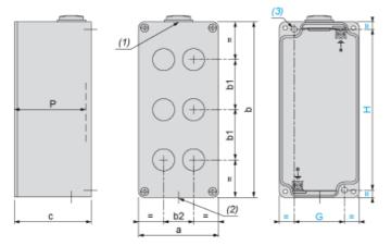
1 hole, with blanking plug (protrusion 6 mm/0.24 in.), for cable gland ISO M25 x 1.5 1 hole, without blanking plug, for cable gland ISO M25 x 1.5 2 x  $\emptyset$  5.6 mm/0.22 in. holes, depth 19 mm/0.75 in.
