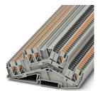
Double-level terminal block, nom. voltage: 800 V, nominal current: 20 A, connection method: Push-in connection, 1st and 2nd level, Rated cross section:  $2.5~\text{mm}^2$ , cross section:  $0.14~\text{mm}^2$  -  $4~\text{mm}^2$ , mounting type: NS 35/7,5, NS 35/15, color: gray
