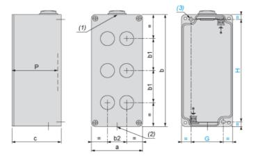
1 hole, with blanking plug (protrusion 6 mm/0.24 in.), for cable gland ISO M20 x 1.5 1 hole, without blanking plug, for cable gland ISO M20 x 1.5 2 x  $\varnothing$  5.6 mm/0.22 in. holes, depth 19 mm/0.75 in.
