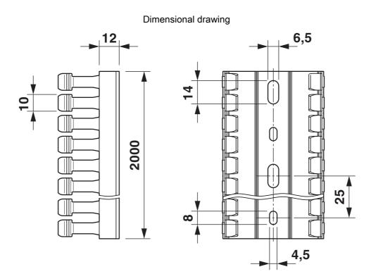
Base perforation according to DIN EN 50085
