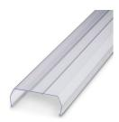
Cover profile for covering terminal strips, snaps onto cover profile carrier APT-ME or end clamp APH-ME. A cover profile carrier is to be positioned at the ends and at intervals of around 40 cm. Length as per customer requirement.
