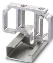
End clamp, for end support of UKH 50 - UKH 240, is pushed onto DIN rail NS 32 and fixed with 2 screws, width: 10 mm, color: Aluminum
