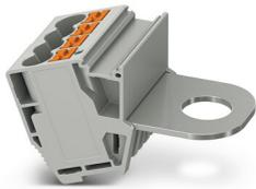
Pick-off terminal, nom. voltage: 1000 V, nominal current: 41 A, number of connections: 5, connection method: Push-in connection, 1 level, Rated cross section: 6 mm<sup>2</sup>, cross section: 0.5 mm<sup>2</sup> - 10 mm<sup>2</sup>, Bolt connection, 1 level, mounting type: on base element, color: gray
