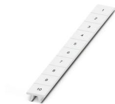
Zack marker strip, Strip, white, labeled, can be labeled with: CMS-P1-PLOTTER, Printed vertically: consecutive numbers 1 ... 10, 11 ... 20, etc. up to 91 ... 100, mounting type: snapped, for terminal block width: 10.2 mm, lettering field size: 10,15 x 10,5 mm, Number of individual labels: 10
