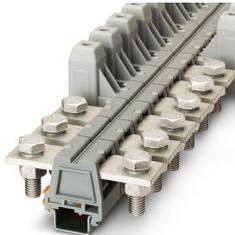
Universal terminal block with bolt connection, cross section: 35 ... 95 mm<sup>2</sup>, AWG: 2 ... 4/0, width: 40 mm, color: gray
