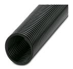
Protective hose, material: PA 6, UV-resistant: yes, flexible, degree of protection: IP68, color: black, flammability rating in acc. with UL 94: V0, inner diameter: 36 mm, Total length: 25 m
