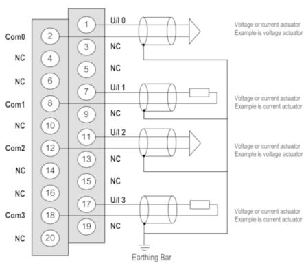
U/Ix + pole input for channel x COMx - pole input for channel x Channel 0 Voltage actuator Channel 1 Current actuator
