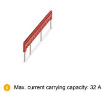
Plug-in bridge, non-adjacent, pitch: 8.2 mm, number of positions: 16, pin assignment: 1, 7, 13, 16, color: red
