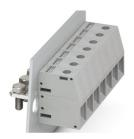
Panel feed-through terminal block, connection method: Screw connection with tension sleeve, Cable lug connection, number of positions: 1, load current: 150 A, cross section:  $16 \text{ mm}^2 - 50 \text{ mm}^2$ , connection direction of the conductor to plug-in direction:  $0^\circ$ , width: 18.8 mm
