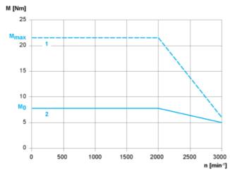
1: Peak torque2: Continuous torque
