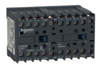
reversing Contactor, TeSys K, 3P, AC-3/AC-3e,440V 9A, 1NC, 48V AC coil, solder pins for printed circuit boards
