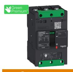
circuit breaker ComPact NSXm B (25 kA at 415 VAC), 3P 3d, 50 A rating TMD trip unit, compression lugs and busbar connectors
