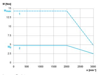
1: Peak torque2: Continuous torque
