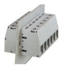
Panel feed-through terminal block, connection method: Screw connection with tension sleeve, Screw connection with tension sleeve, number of positions: 1, load current: 150 A, cross section: 16 mm<sup>2</sup> - 50 mm<sup>2</sup>, connection direction of the conductor to plug-in direction: 0 °, width: 18.8 mm
