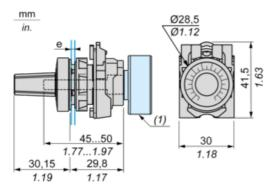
$\boldsymbol{e}\text{:}$  clamping thickness: 1 mm to 6 mm / 0.03 in. to 0.24 in.
