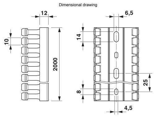
Base perforation according to DIN EN 50085
