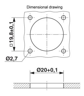
Installation dimensions Flat gasket, radial O-ring
