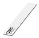
Marker for terminal blocks, Card, white, unlabeled, can be labeled with: Marker pen, perforated, mounting type: snap in, snap into flat marker groove, for terminal block width: 7.5 mm, lettering field size:  $15 \times 7.5 \text{ mm}$ , Number of individual labels: 10
