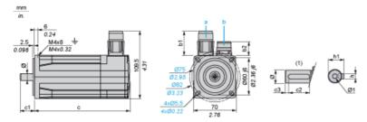
a: Power supply for servo motor brake
